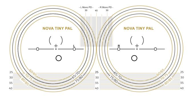
Fitting cross is located 3mm above lens Prism Reference Point.
